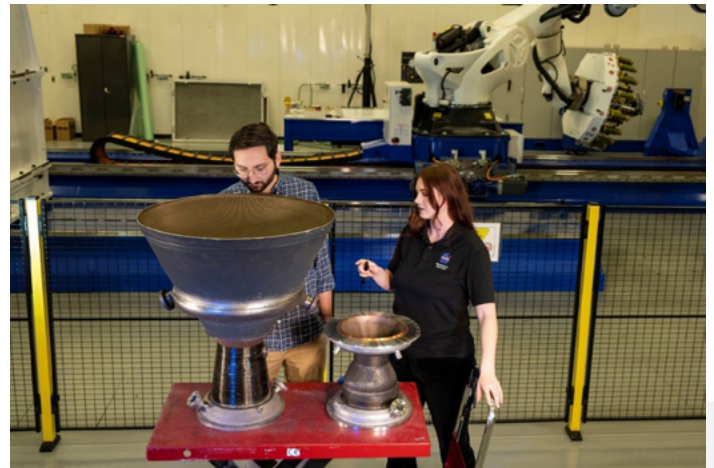
Figure 15: Project engineers at NASA’s Marshall Space Flight Center in Huntsville, Alabama, inspect an additively manufactured composite overwrap thrust chamber assembly. (Credit: NASA)
