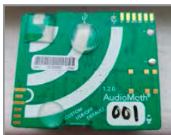
AudioMoth made tactilely accessible with bump dots
